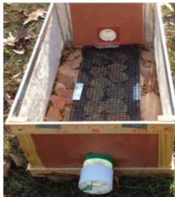
Figure 7. Two-fan trap designed by MacHardy, actual trap with leaves on the left, schematic showing design on the right. (W.E. MacHardy)
