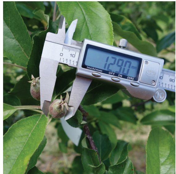
Figure 3. Measuring fruit diameter with electronic calipers.
