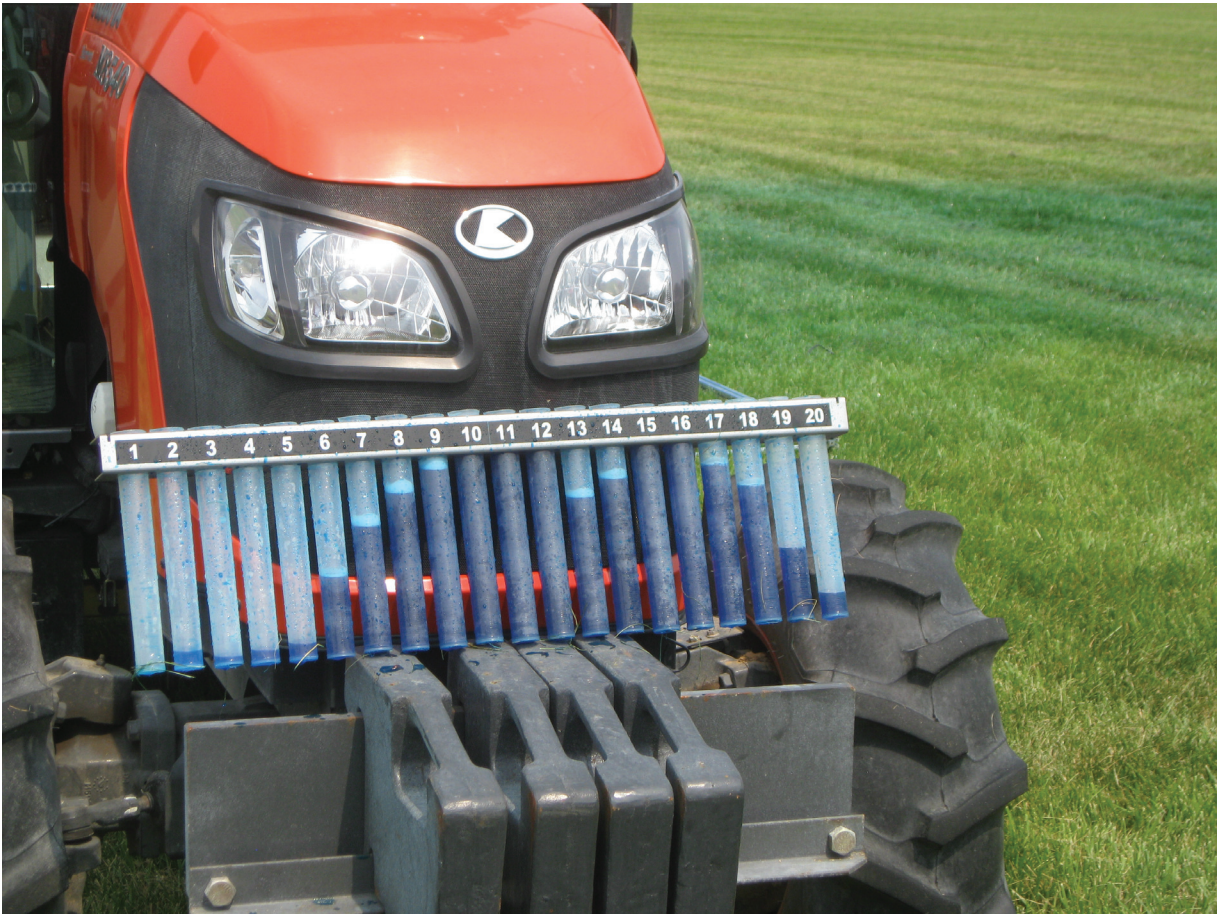
The collected water (here died blue) visually demonstrates the pattern of application from the lowest collector (right) to the highest collector (left).
